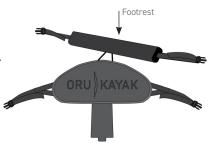
Stern bulkhead: Provides structural rigidity.
