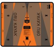
6 Stern (rear) floorboard: Reinforces kayak bottom and holds the rear and middle seat.
